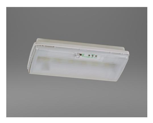
A self testing, high output LED with frosted diffuser, emergency bulkhead. The X-RSL3M tests the battery voltage and LED output regularly and signals the results so that you can easily maintain your testing records. For internal environments this low profile unit can be fitted with a suspended legend kit to create a emergency exit sign.
