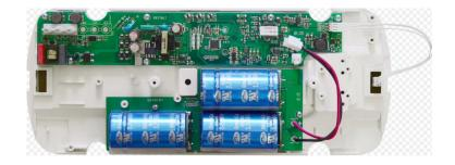
Robust Bulkhead for heavy duty cold storage refrigeration applications. The X-SZ1M/SC has a power pack consisting of super capacitors and not conventional batteries.
